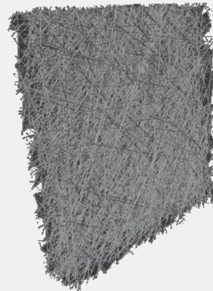
Virtual filter medium microstructure
