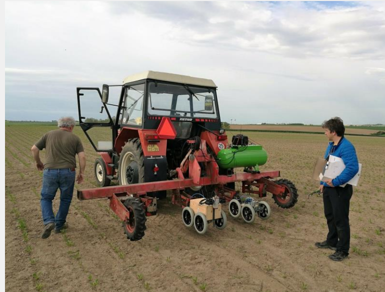
Agricultural weeding machine device for recognition of the target crop from weed.
