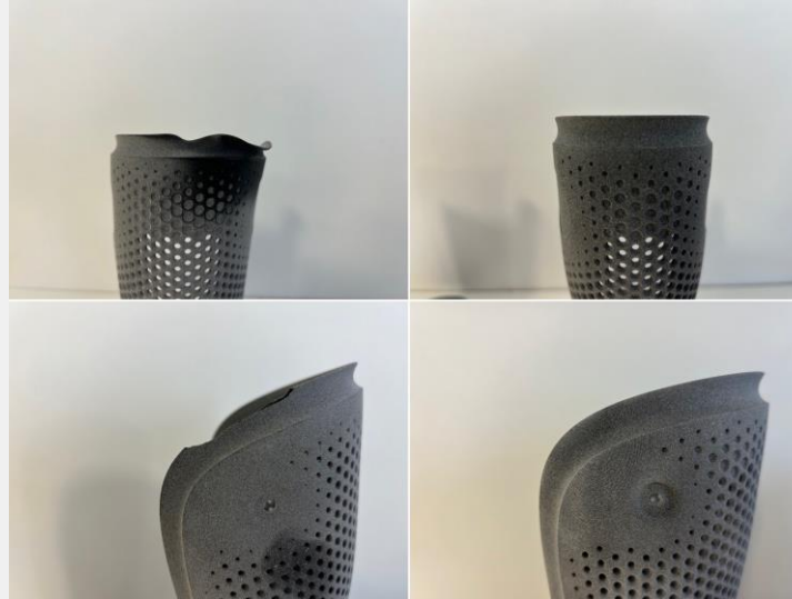
The first column shows two different types of product deformation. As you can see, the shape of the product is damaged. The next column shows the final product that meets the quality standards.
