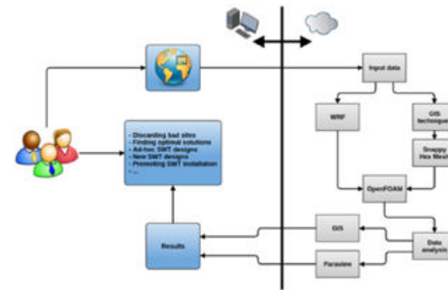
Workflow diagram representing the interaction between Cloud computing software solution and users/decision makers for wind-turbine position optimization
