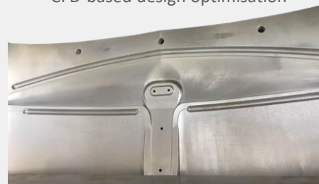
Hydrofoil mold used to create a prototype design.
