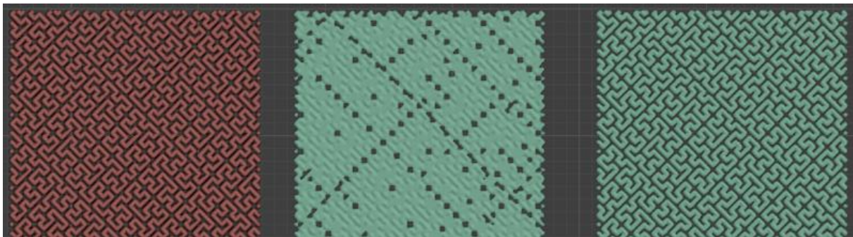
Figure 11 – 80% Hilbert Curve lattice – from left: original, voxel size 0.1 mm, voxel size 0.05 mm
