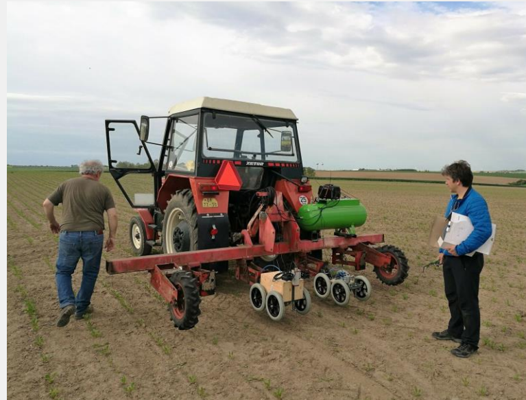
Agricultural weeding machine device for recognition of the target crop from weed.
