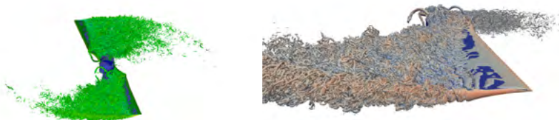
Figure 1: Visualisation of the vortical structures in the flow around the "Iowa" rotor at Reynolds number 15000 for the whole rotor (left) and zoom in to the blade tip (right). Flow complexity and the wide range of the vortex scales are clearly visible.
