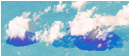
Figure 3: 3D visualization of simulated convective clouds by DALES. Clouds are shown in white and rain is shown in gray. The air temperature near the surface is shown in blue, dark blue areas being cold pools associated with rain. By Johanna Grönqvist and Fredrik Jansson, TU Delft.
