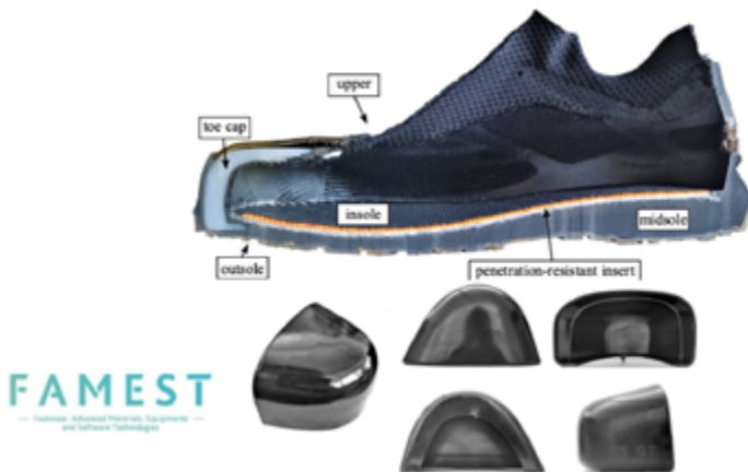
Figure 2: Optimized molds that resulted from the simulations
