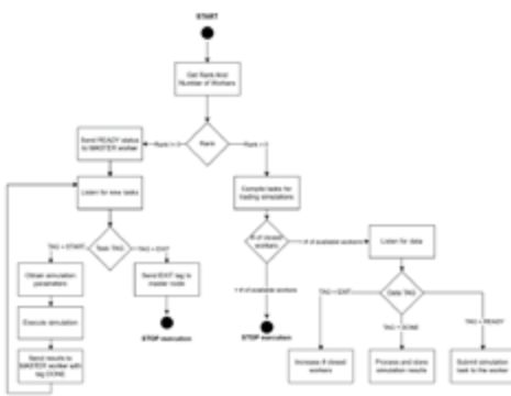
Figure 1: Orchestration of trading simulations for multinode multicore environment
