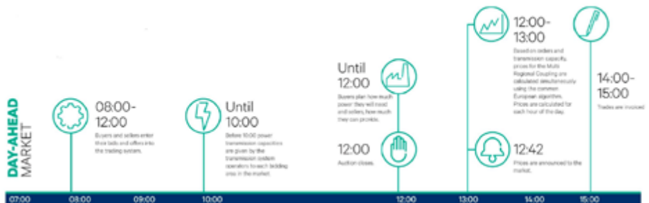
Figure 1: Day ahead trading market with time critical window of operation between 10:00 and 12:00. © SINTEF ENERGY
