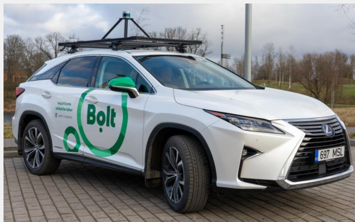
Lexus RX450h equipped with the sensors that are a prerequisite for basic autonomy.
