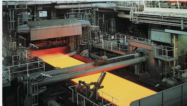
Illustration of the steel sheet cooling process.
