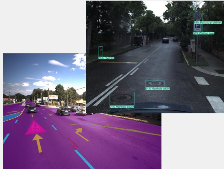
Image processing results on ground survey images, from which spatial data can be generated.
